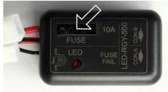
2) Carefully open the cover. Be careful to don't damage the fixing pins on the corners !!!
